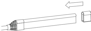
Apply waterproof glue to the end cap, then install the cap.
