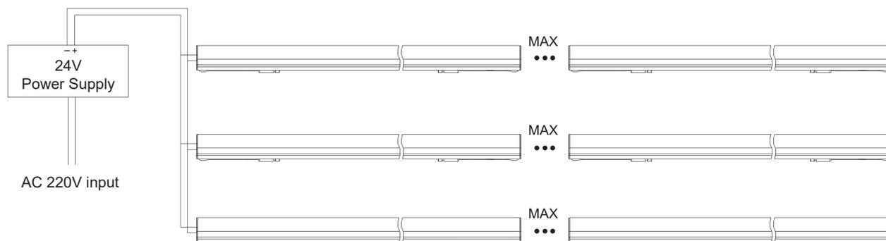
Note: the "MAX" here means the max connectable series
